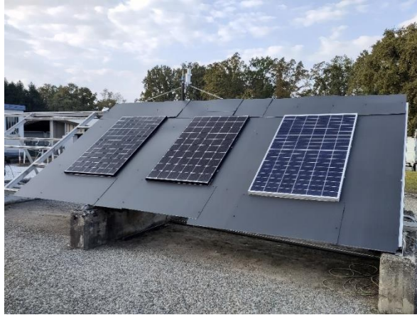
Figure 28. Installation of module operating temperature measurements according to the IEC 61853-2:2016 at the ESTI outdoor monitoring test site.
