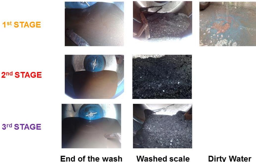
Figure 28. Washing Process Stages
