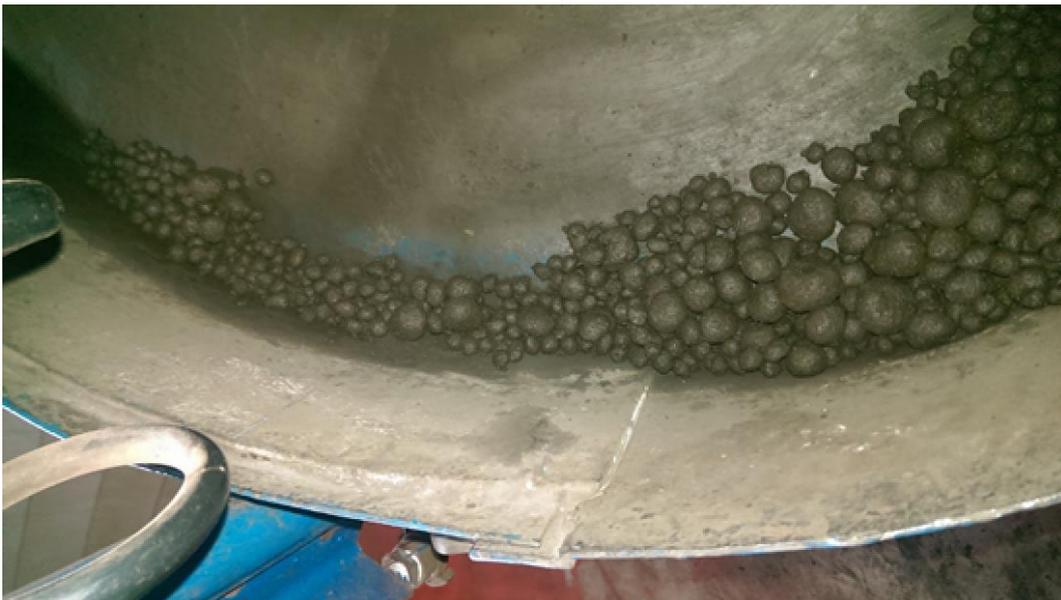
Figure N12: High quality pellets produced following the "winning formula".
