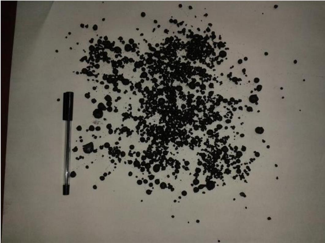
Figure N11: Low quality pellets produced with the mixture composition n° 1.
