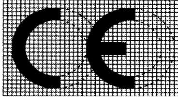
2. If the CE marking is reduced or enlarged the proportions given in the above graduated drawing shall be respected.
