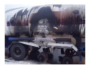
Transport vehicle tyre fires mainly occur when travelling on highways, but can also break out when parked after travelling.
