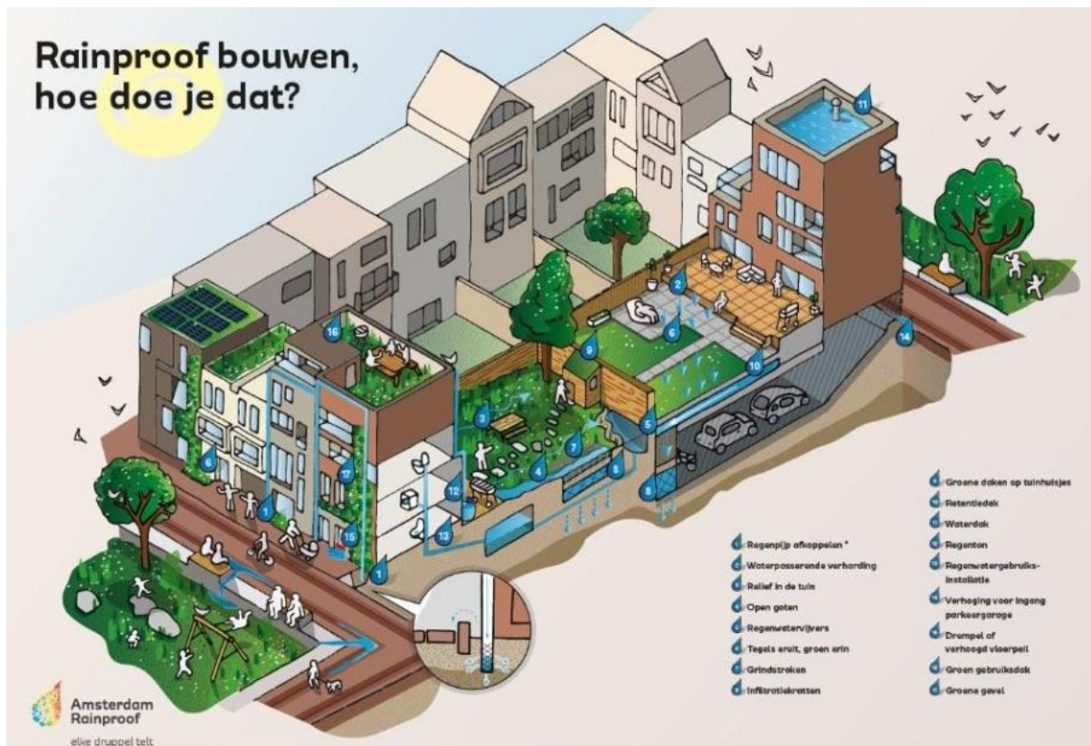
Figure 17. Integrated rainwater management at building plot level.
