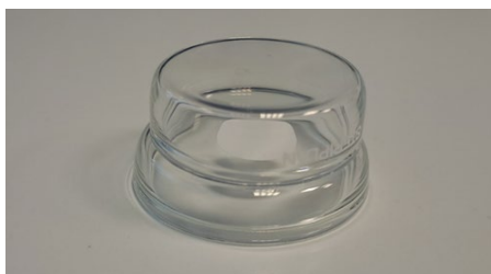
Annex II Figure 2 Alumina filter placed on top of a Petri dish turned upside down and covered by the bottom part of the dish
