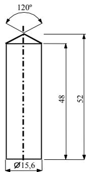
Fig.2: Cylindrical bronze piston, dimensions in mm
