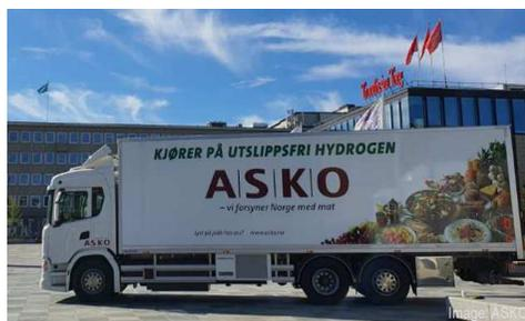
**Brief description:** FCH HD trucks use an electric motor powered by a fuel cell, combined with a battery (hybrid powertrain)
