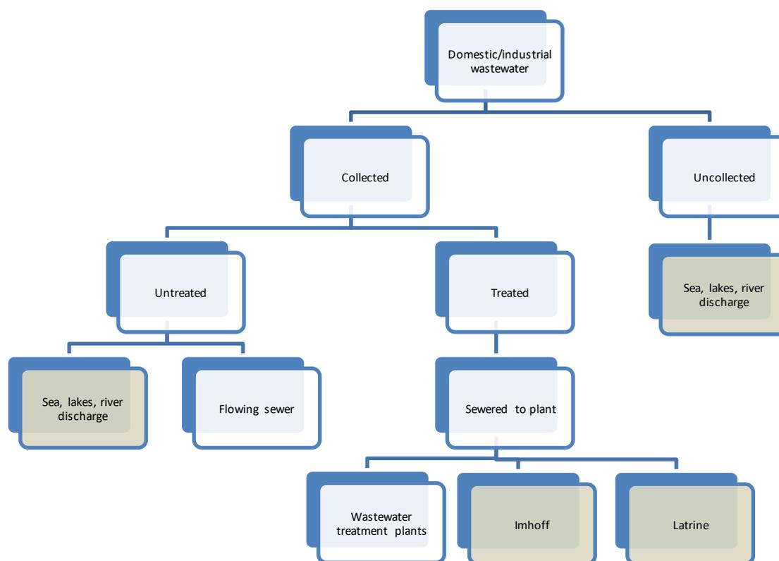
Figure 7.6 Domestic wastewater treatment system and discharge pathways
