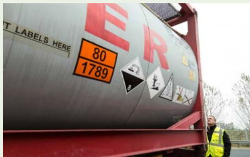
The orange plate displayed at both the front and the rear of a vehicle informs about the type of hazard and the substance carried. The number 80 in the upper half of the orange plate stands for “corrosive or slightly corrosive substance”, while the number 1789 in the lower half stands for “hydrochloric acid”.
