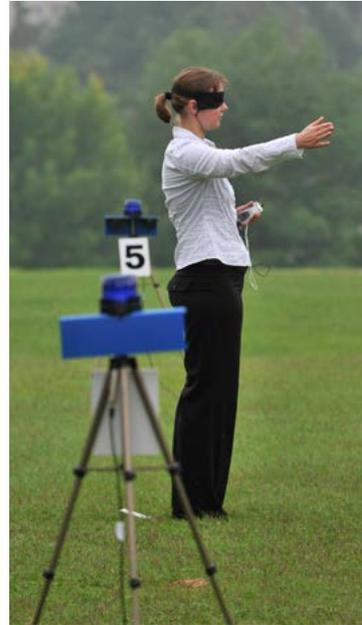
A UNECE ITC WP.29 demonstration of sound devices that "silent cars" could be equipped with
