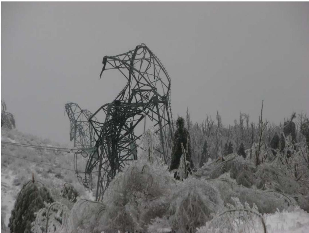
FIG.4. Damage caused by glaze ice on the 400 kV powerline Beričevo-Divača in Slovenia, February 2014. Courtesy of ELES (Slovenian transmission network operator) [81].
