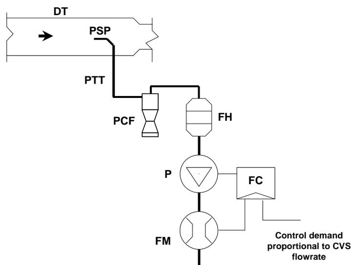
A sample of the diluted exhaust gas is taken from the full flow dilution tunnel DT through the particulate sampling probe PSP and the particulate transfer tube PTT by means of the pump P. The sample is passed through the particle size pre-classifier PCF and the filter holder(s) FH that contain the particulate sampling filter(s). The flow rate for sampling is set by the flow controller FC.
