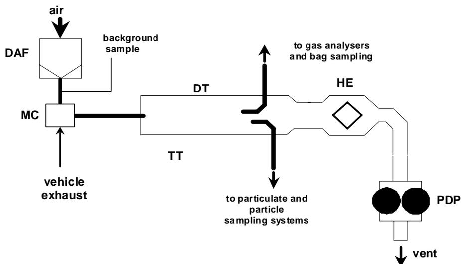
The positive displacement pump (PDP) full flow dilution system satisfies the requirements of this annex by metering the flow of gas through the pump at constant temperature and pressure. The total volume is measured by counting the revolutions made by the calibrated positive displacement pump. The proportional sample is achieved by sampling with pump, flowmeter and flow control valve at a constant flow rate. The collecting equipment consists of:
