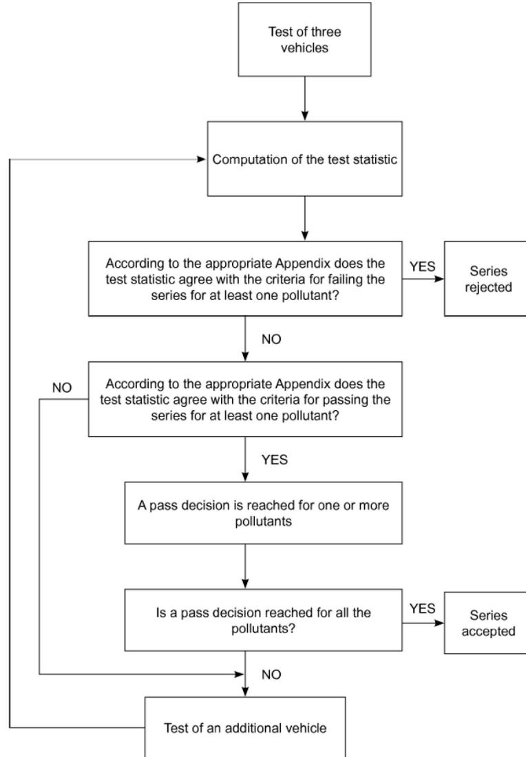
8.2.3. Notwithstanding the requirements of paragraph 5.3.1. of this Regulation, the tests shall be carried out on vehicles coming straight off the production line.
