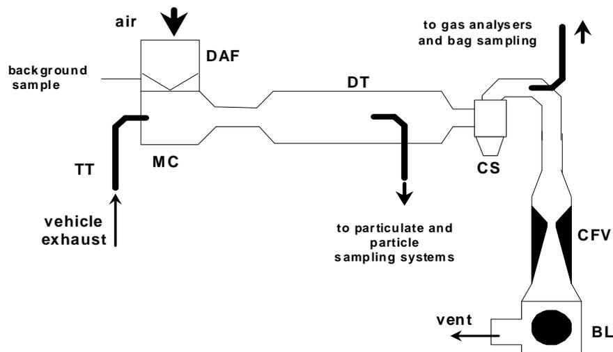
The use of a critical-flow venturi (CFV) for the full-flow dilution system is based on the principles of flow mechanics for critical flow. The variable mixture flow rate of dilution and exhaust gas is maintained at sonic velocity which is directly proportional to the square root of the gas temperature. Flow is continually monitored, computed and integrated throughout the test.
