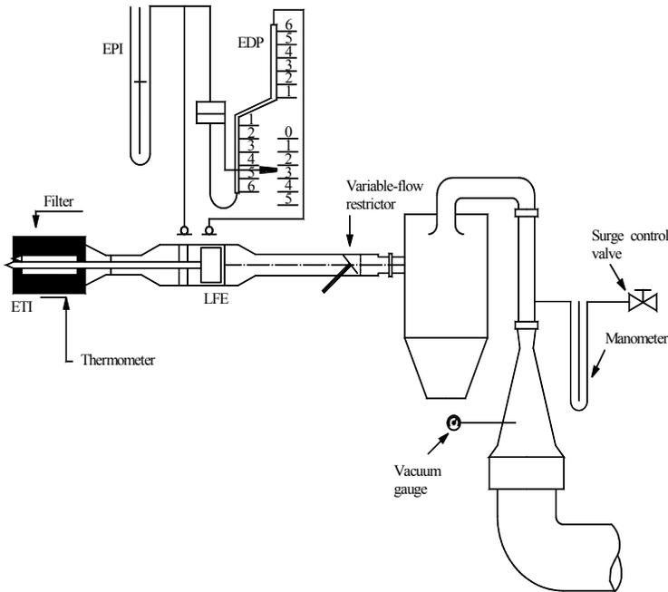
2.3.5. The variable-flow restrictor shall be set to the open position, the blower shall be started and the system stabilized. Data from all instruments shall be recorded.
