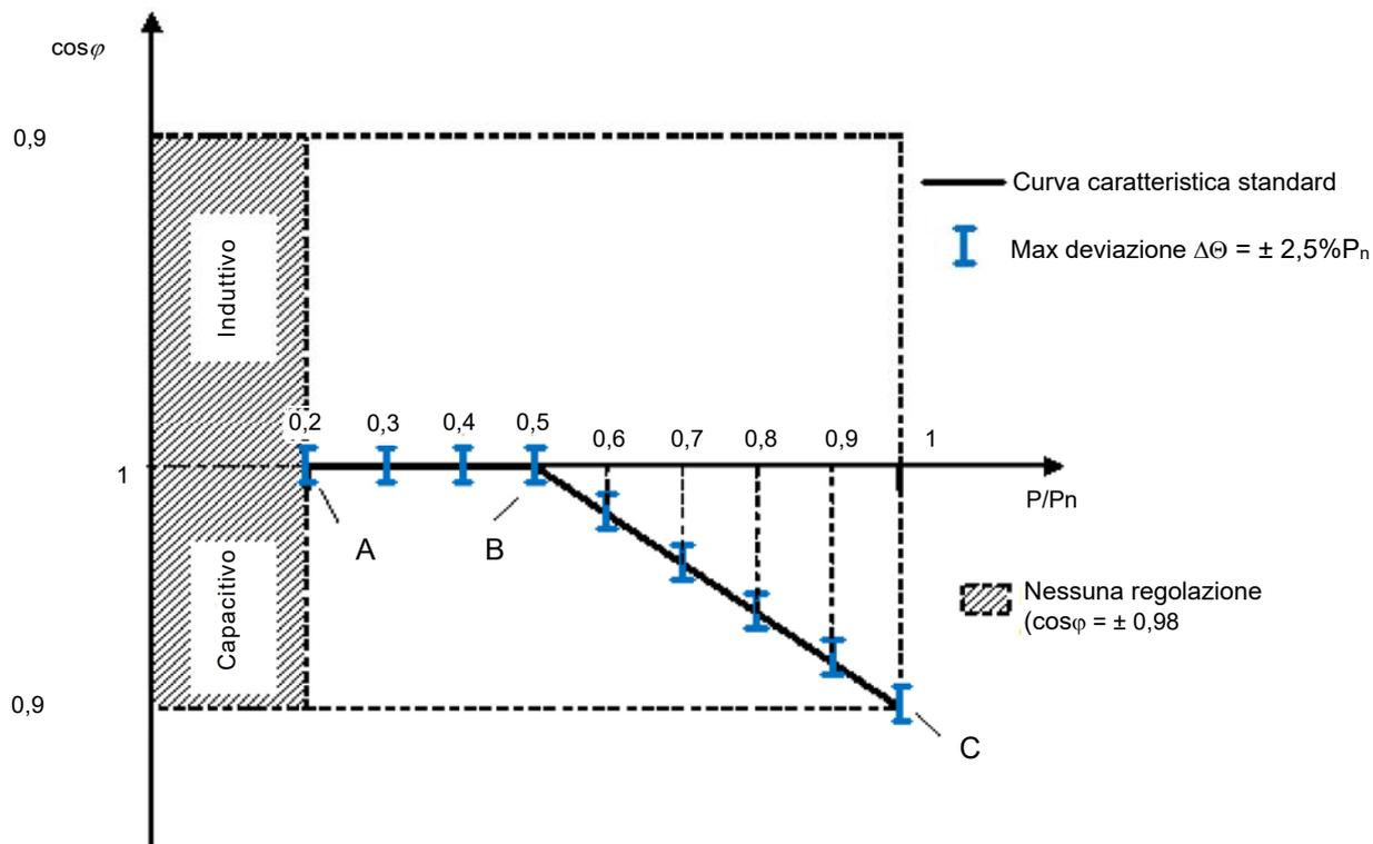
**Figura 27 – Curva caratteristica standard  $\cos\varphi = f(P)$**
