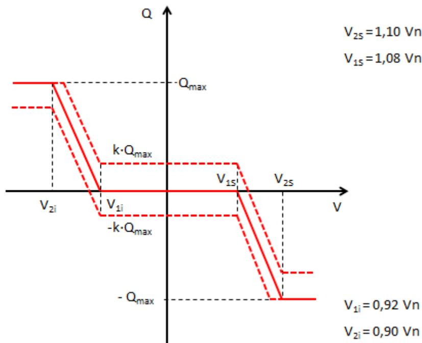
**Figura 39 – Curve caratteristiche standard  $Q = f(V)$  <sup>(87)</sup>**
