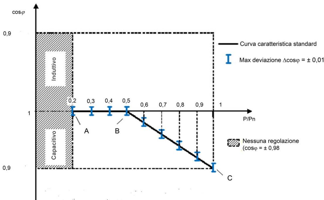
**Figura 7Bbis – Curva caratteristica standard  $\cos\varphi = f(P)$**
