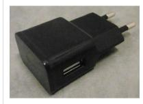
Travel Adapter Model: DT-09T Input: ACIO-240 - 0.35A 50-60Hz Output: DC 5.0V == 1A C C D D D For Indoor use only Made in China Alert number: A12/1314/18 Product: Battery charger Name: Nuprol Lipo 3 Risk type: Electric shock Category: Electrical appliances and equipment Brand: Nuprol Ltd Type / number of model: Lipo 3 Risk level: Serious risk The electrical insulation is inadequate. As a result, accessible parts can become live and the user could receive an electric shock from them.
