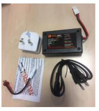
Alert number: A12/1317/18 Product: Battery charger Name: Lipo Battery charger Risk type: Electric shock Category: Electrical appliances and equipment Brand: Nuprol Ltd Type / number of model: SM4 Risk level: Serious risk The electrical insulation is inadequate. As a result, accessible parts of the product could become live. The user could receive an electric shock from them.
