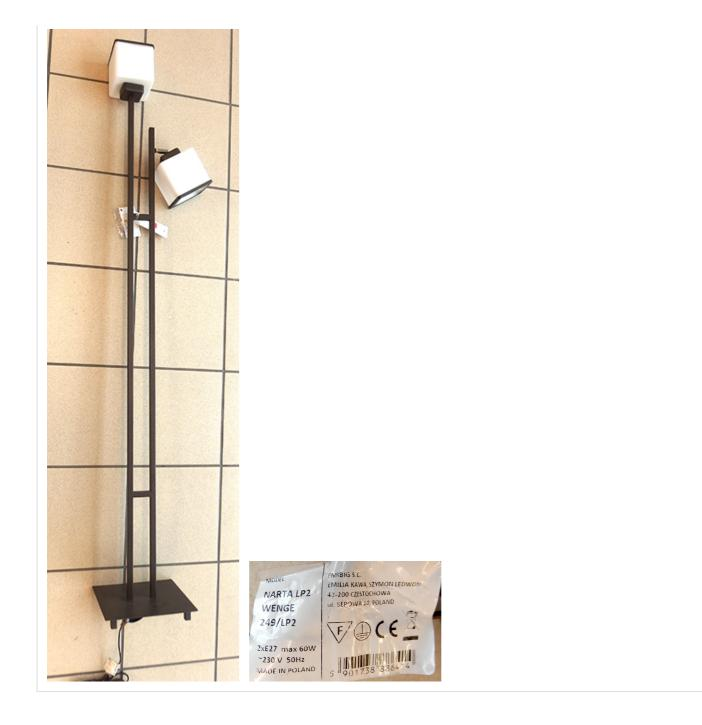
Alert number: A11/00003/20 Product: Floor lamp Name: Risk type: Electric shock Category: Lighting equipment Brand: EMIBIG Type / number of model: Bingo LP2 727/LP2 Type of alert: Products with other risk levels The insulation between the cables and the external metal housing (which has sharp edges) is inadequate.
